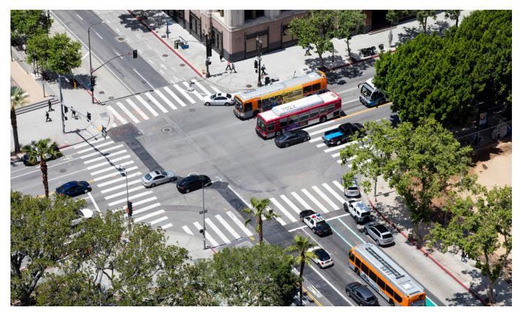
Traffic lights at intersections are managed by simple computers that assign the right of way to the nonconflicting direction. However, studies looking at travel times in urban areas have shown that delays caused by intersections make up 12-55% of daily commute travel, which could be reduced if the operation of these controllers were made more efficient.
